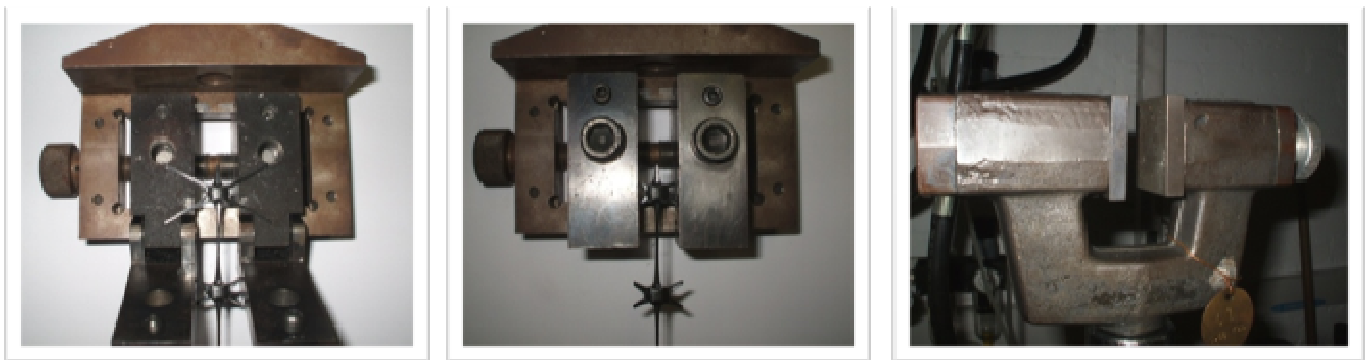
Figure 6- typical example of 'Junction strength' test clamps (6a & 6b show the upper junction clamp in open and closed positions; 6c shows the lower node/junction clamp)
