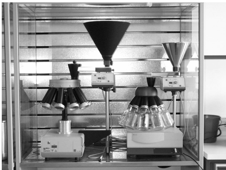
Figure 24: Sample divider with eight portions (Retsch DR 100, left) and sample divider with ten portions (Fritsch Laborette 27, right).
